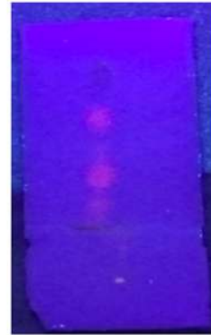
Figure 1: Thin Layer Chromatographic separation of methanolic extracts of the plant. 3 spots were identified with good separation
