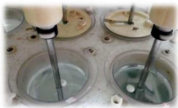
Fig.1 In vitro buoyancy of Venlafaxine HCl floating tablets
