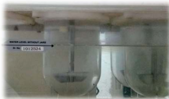
Fig.2: In vitro dissolution of venlafaxine HCl floating tablets
